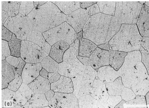
Figure 5 Optical microstructures of as-forged, rolled and water-quenched samples along longitudinal direction shows grain growth in all cases: (a) unmodified, (b) boron-modified, and (c) the least being in (B + Ti)-modified alloy. \times 150 .
